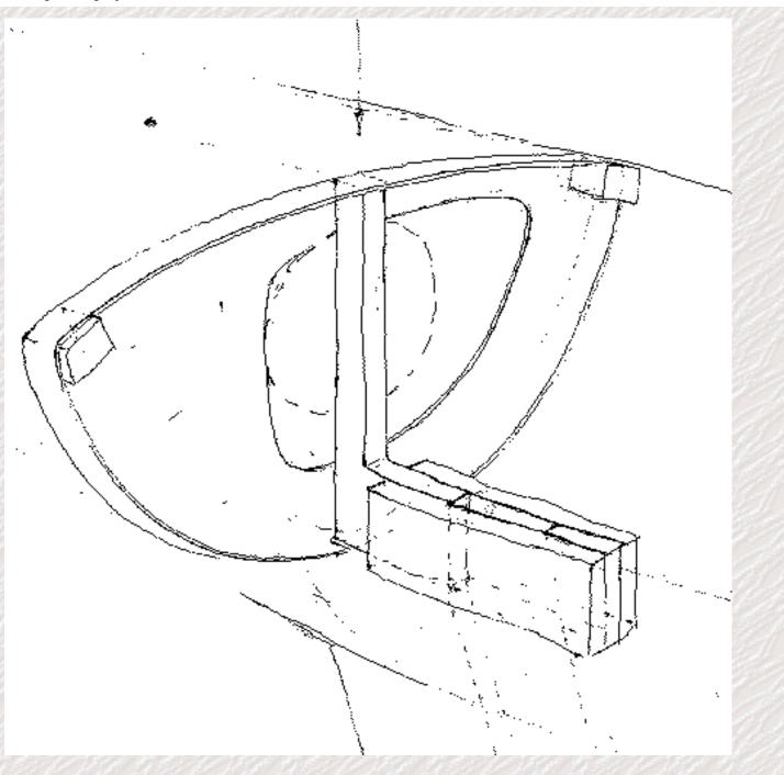
Note that the above drawing does not show the "new" bulkhead style (1997) which has a little "dip" in the center to clear a small mast support block. The presence of this block will certainly help, but in my opinion, will not solve the long term load problems at this position.
